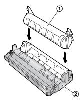
**8** Firmly press down the toner cartridge to snap into position (1).
